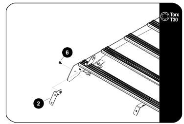
Secure the Wind Fairing Side Supports LH / RH (Item 2) to the foot rails bottom holes as shown using M6x16 Flange Button Head (Item 6).
