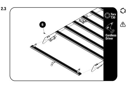
Secure assembly 2.2 to the front two top holes on the foot rails using the fasteners supplied with KSSX001.
