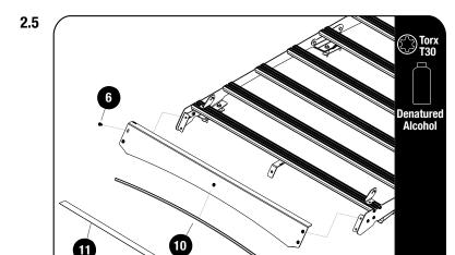
Fit the Wind Fairing Rubber (Item 10) to the Light Bar Wind Fairing (Item 1). Using the notched section as a guide, trim if needed.
