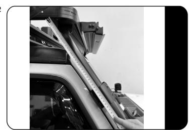
C) Loosen the nut securing the Pillar Bracket to the underside of the Rack before continuing to the next step.
