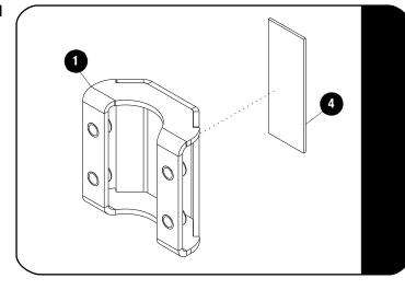
Clean the rear of the Back Bracket (Item1) with Denatured alcohol and adhere the VHB tape (Item 4) to the back of the Mounting bracket.
