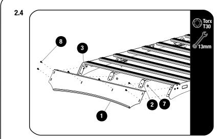
Secure the Wind Fairing (Item 1) first to the Side Bracket Assemblies (Item 3), using M6 x 16 Button Head Flange Bolts (Item 8).
