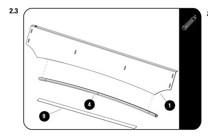
Fit the Wind Fairing Rubber (Item 4) to the Wind Fairing (Item 1). Using the notched section as a guide, trim if needed.
