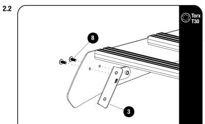
Secure the Side Bracket Assemblies LH & RH (Item 3) to the foot rails bottom holes as shown using M6 x 16 Button Head Flange Bolts (Item 8).
