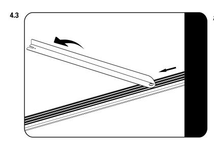
Slide the nut assembled to the Wind Deflector into the T-slot of the Narrow Slat as shown.
